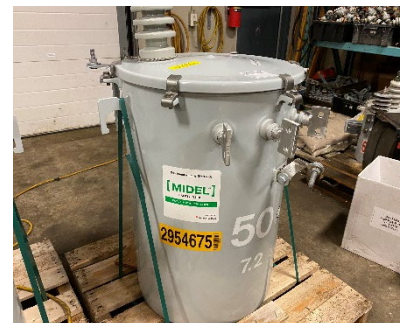
A distribution transformer containing synthetic biodegradable ester.
